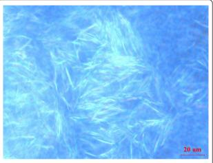
Figure 3 Photo of paraffin crystal in simulated crude oil.
