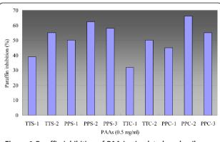
Figure 1 Paraffin inhibition of PAA in simulated crude oil.
