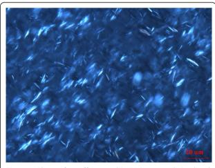
Figure 4 Photo of paraffin crystal in PPC-2 treated simulated crude oil.
