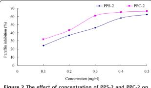
Figure 2 The effect of concentration of PPS-2 and PPC-2 on the paraffin inhibition.
